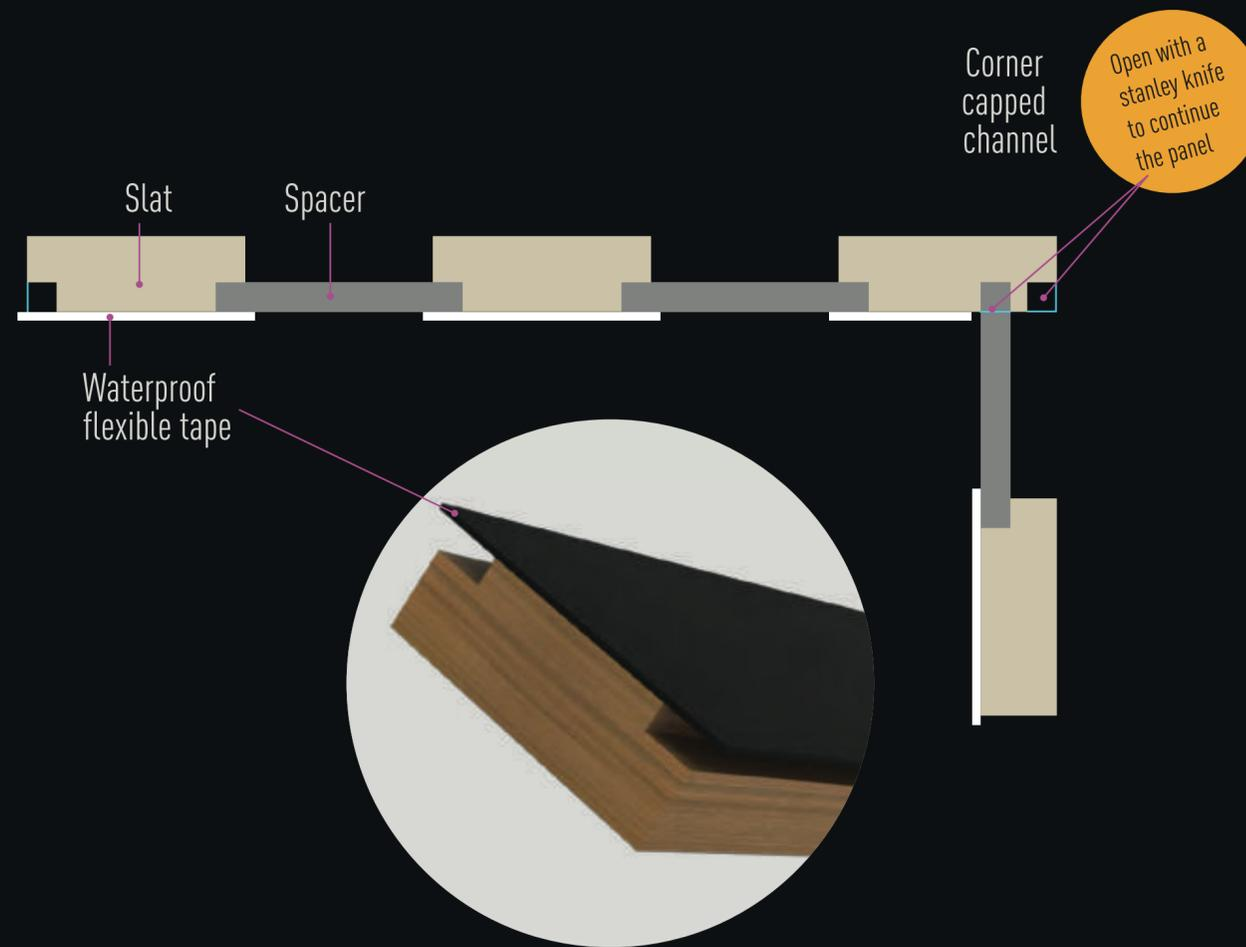
**FLEXIBLE TAPE + MDF + SPACER = FLEX SLATTED**
